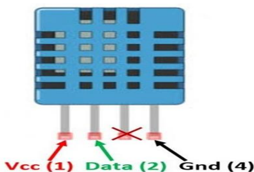
Fig: 4: DHT11 (Humidity and temperature) sensor
